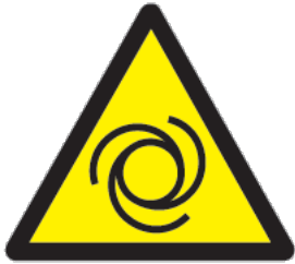
Machinery starts automatically
